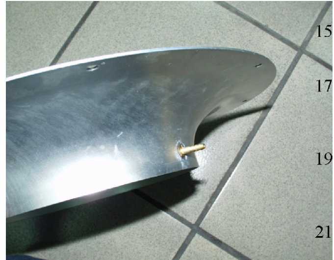
Fig. 5. Pressure sensor installed at the entrance of the FFU inlet mouth.
